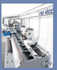
The machine takes its name from the four guideways along which the slides, tailstock and steady rest are moved. Precise, anti-friction bearings on a heavy-duty and torsion-resistant bed ensure the utmost positioning accuracy of the bed slides. The tailstocks and steady rest are precisely guided on hardened and finely-ground steel rails that are screwed on to the machine.
