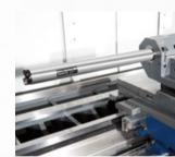
The design provides the straight-forward and precise change-over of the various tooling systems that range from tool turret, boring block and milling attachment through to a grinding unit on a quick-release plate.
