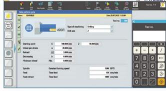
Geometry data screen "groove" (lateral surface)
