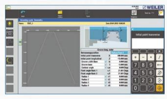
Geometry input – standard geometry
