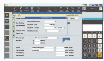
Cutting cycle – extended parameters for machining
