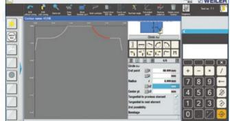
Geometry input – free groove contour
