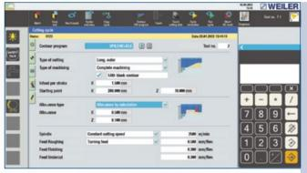
Cutting cycle – various parameters for machining
