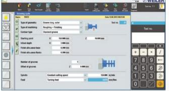
Grooving cycle – various parameters for machining
