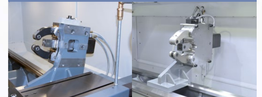
Self-centring follower rest, hydraulically actuated
