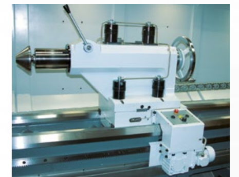
Tailstock with automated clamping and dedicated drive
