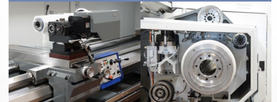
Tool holder head for turning, drilling and milling
