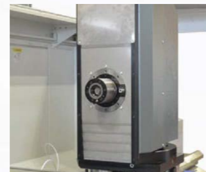
200 mm stroke Y-axis (only with E110/E120)
