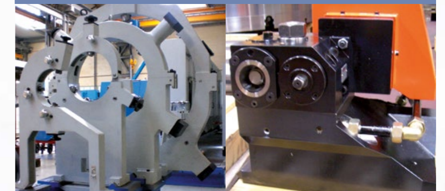
Steady rests for diameters up to 1,500 mm
