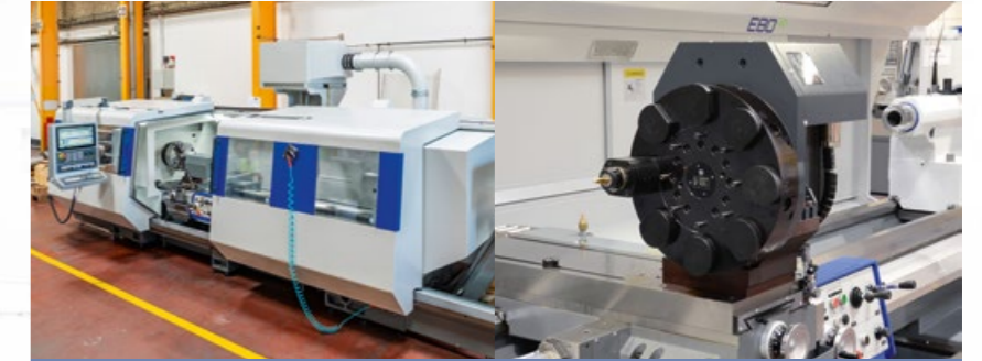
8 station disk turret with driven tools, 40 mm shank diameter
