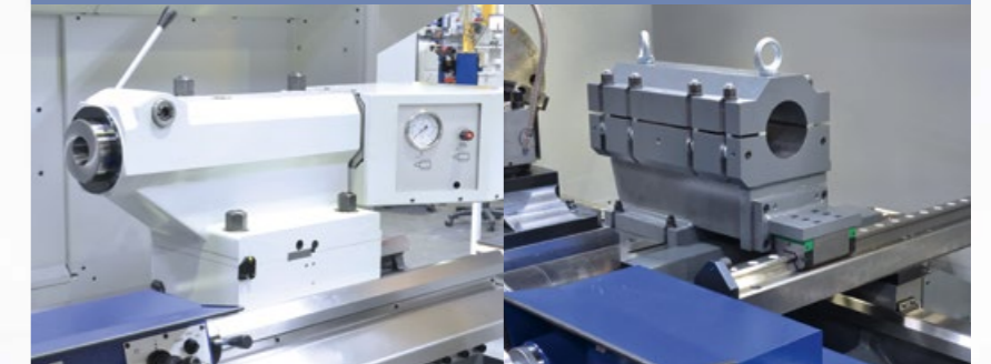
Tailstock with hydraulically actuated quill
