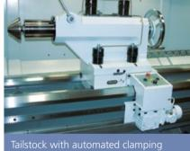
Tailstock with automated clamping and dedicated drive
