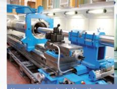
Heavy-duty boring bar holder with additional support and 160 mm bore
