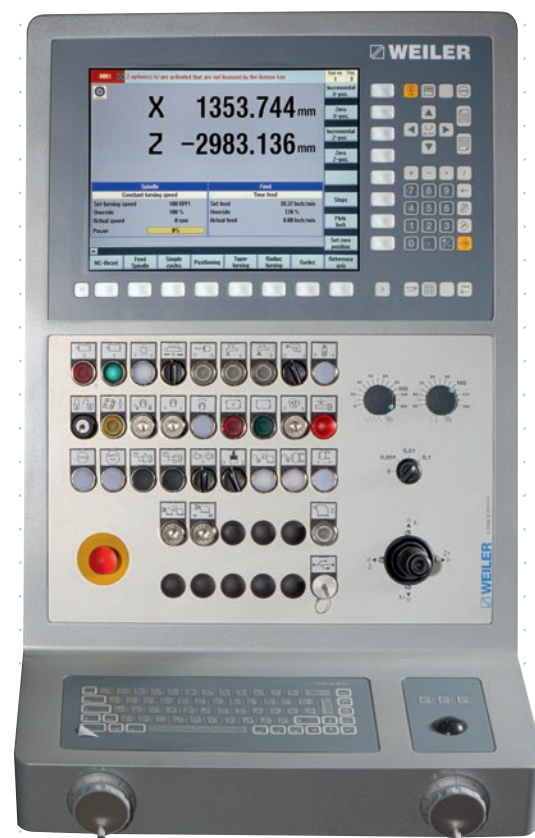
15" screen and additional membrane keyboard with short-stroke keys
