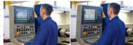
Swivelling control console, standard on all E-series machine tools: dazzling effect eliminated
