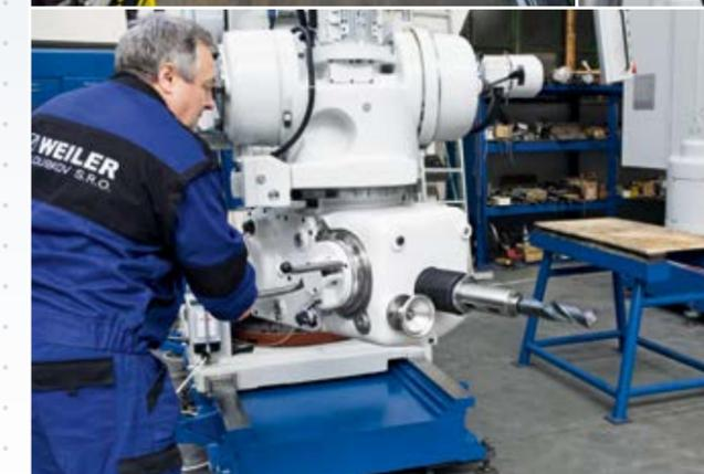
WEILER Holoubkov: assembly of a radial drilling machine
