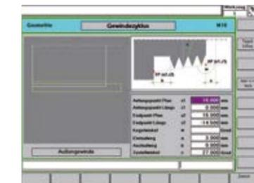
Only a few items of data are needed when entering the thread geometry.
