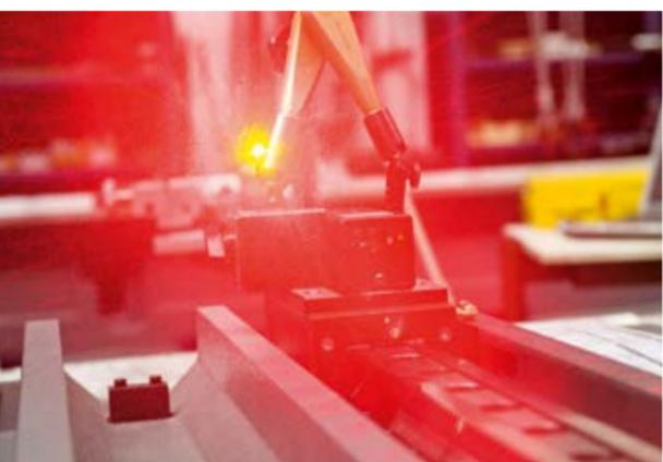
State-of-the-art laser measuring techniques are used to check the guideways.
