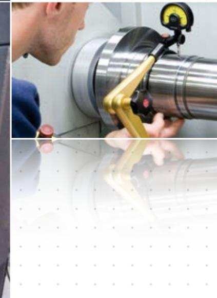
Measuring concentricity. WEILER's production facility ensures that tolerances to the nearest  $\mu$ -metre are achieved.
