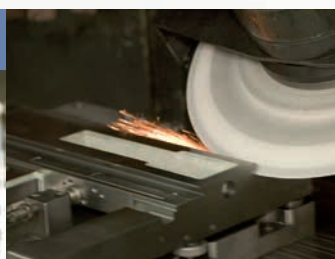
Grinding the dovetail guides
