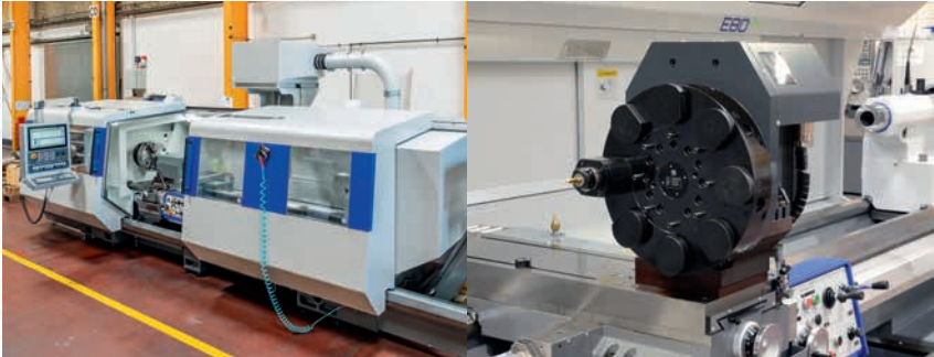
8 station disk turret with driven tools, 40 mm shank diameter
