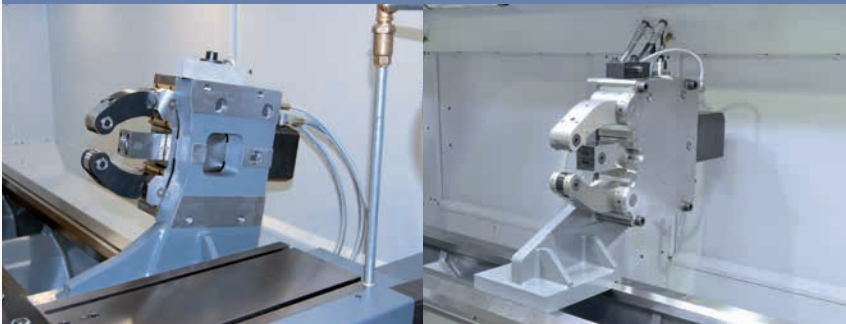
Self-centering follower rest, hydraulically actuated
