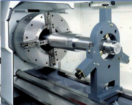
Pneumatically actuated front-end chuck with steady rest
