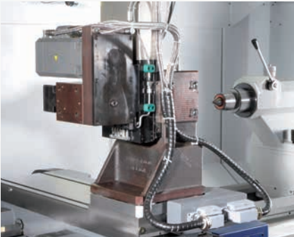
200 mm stroke Y-axis (only with E110/E120)
