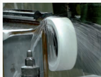
Grinding a machine bed
