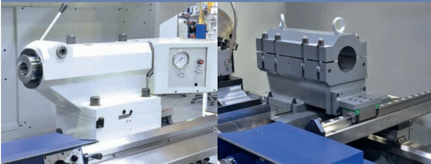
Heavy duty boring bar holder with additional support
