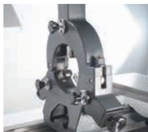
Steady rest with roller jaws Ø 12 – 150 mm
