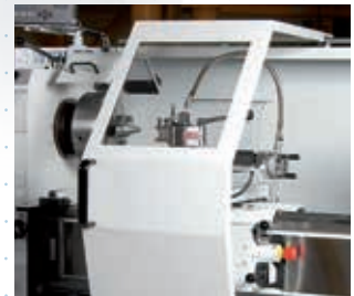
Moveable hood with safety glass pane
