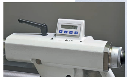
Digital readout for tailstock quill
